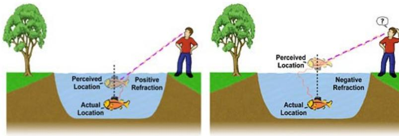
An illustration of how a fish in water is seen by an observer, with the red lines marking the refraction of light and the purple lines representing the path towards the perceived location of the fish, which appears above its actual location. [Print-quality images available for download](#)
