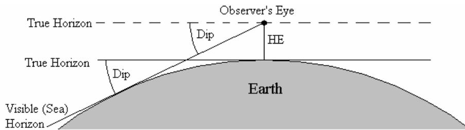
**Figure 5.8** The visible sea horizon is dipped below the true horizon.
