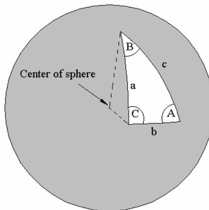
**Figure 4.1** A spherical triangle on the surface of a sphere.
