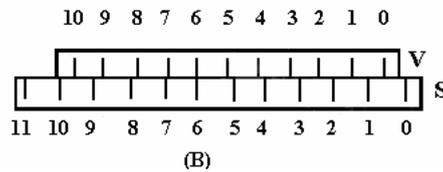
**Figure 5.7** Vernier scale: showing subdivisions of a main scale.
